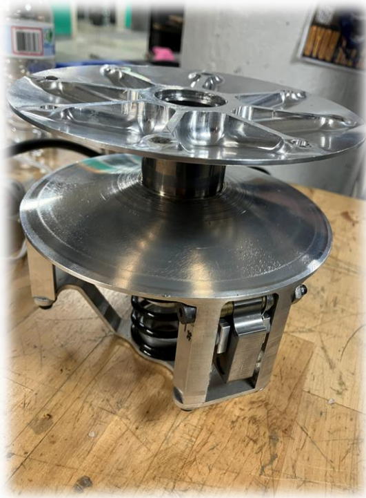
Wear rings from belt on sheaves indicate how far CVT shifted
